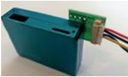
Figure 9. Connecting printed circuit board to Plantower sensor
